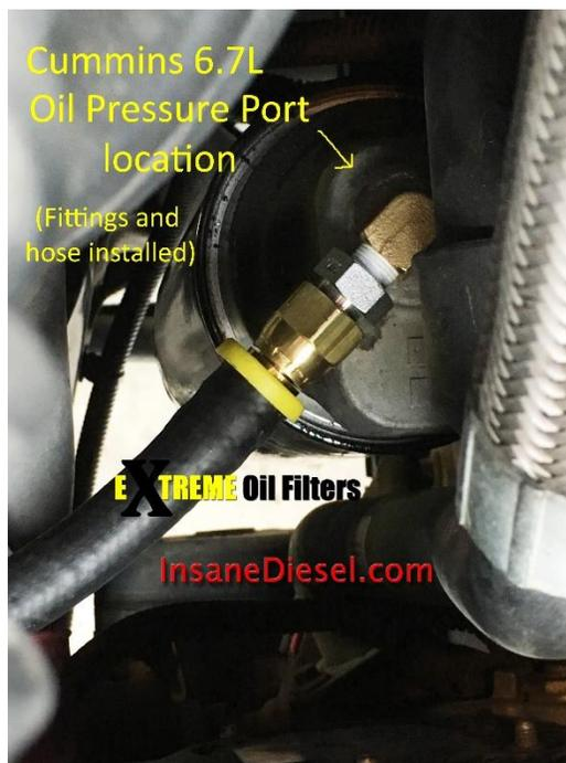
Note: 5.9L location is almost exact same and 6.7L but usually the elbow adaptor is not needed, just the straight adaptor fitting. See picture at end of document
